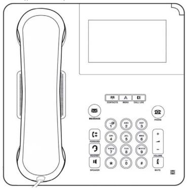
The phone supports 24 programmable call appearance/feature buttons. The labels for these are displayed in the main display and can be controlled by the adjacent buttons.
